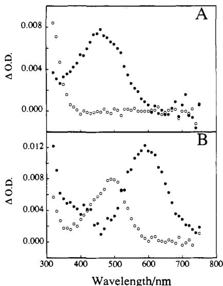
**Figure 1.** Absorption spectra of (A) *tert*-butoxyl (O) and benzyloxyl (●); (B) cumyloxyl (O) and *p*-methoxycumyloxyl (●). The spectra were obtained by 266-nm LFP of di-*tert*-butyl peroxide, dibenzyl hyponitrite, dicumyl peroxide, and bis(4-methoxycumyl) hyponitrite in CH<sub>3</sub>CN, 56, 70, 63, and 61 ns, respectively, after the laser flash. Spectra were recorded under similar, but not standardized, conditions.
